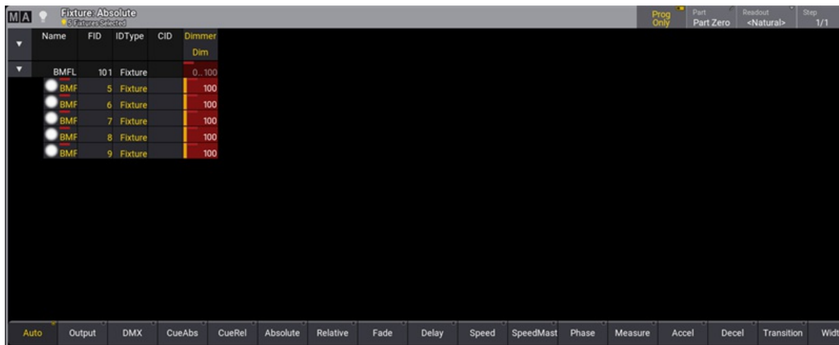
Fixture sheet displaying values for part 1 (Dimmer) with a stronger and brighter red background color.
